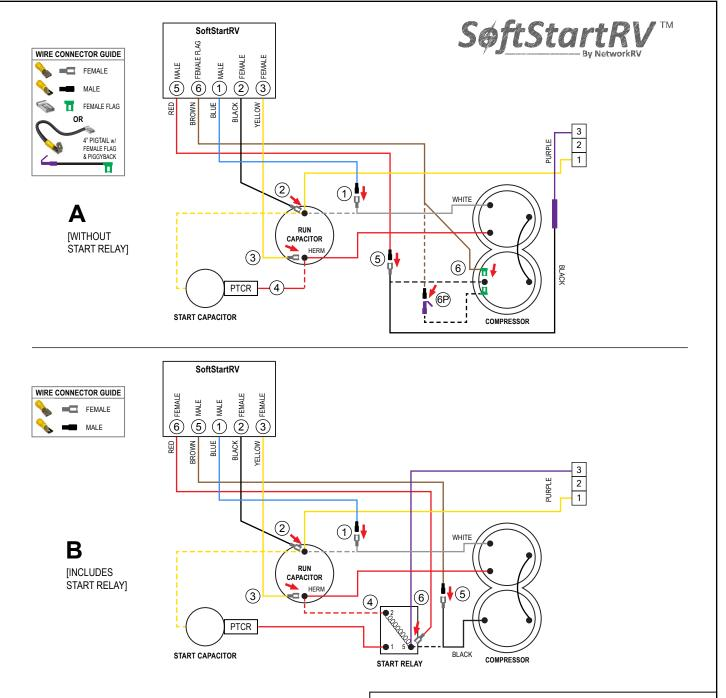
SoftStartRV Wiring Diagram for Coleman Mach 1976D136 (4-09)
