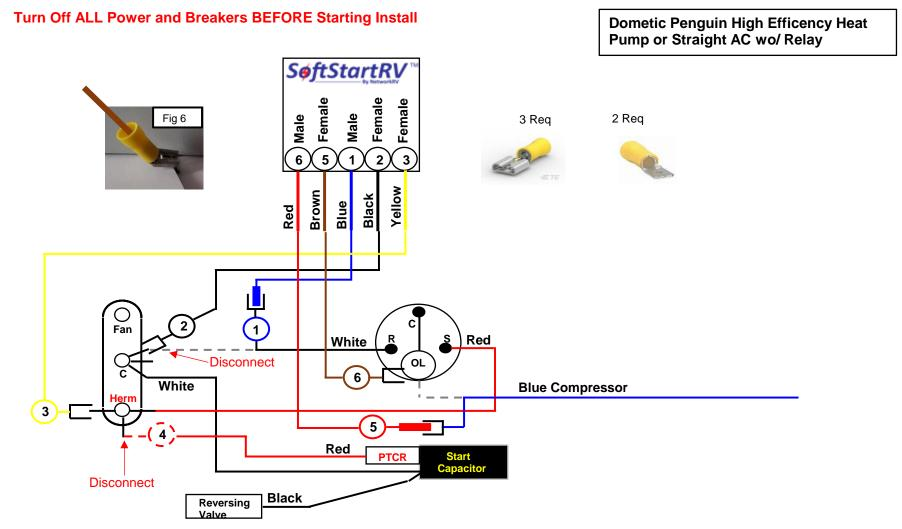
Route Blue, Black and Yellow Softstart wire into Ele Box, Route Brown and Red Softstart wires to top of compressor Crimp disconnects on wire as shown in Softstart box above
