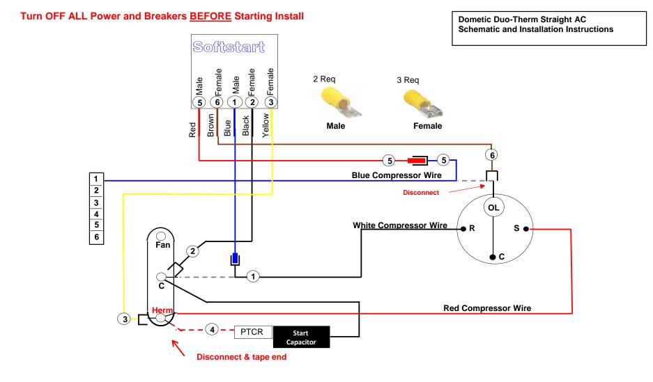
Route Blue, Black and Yellow Softstart wire into electrical Box and crimp disconnect as shown in softstastr drawing above
