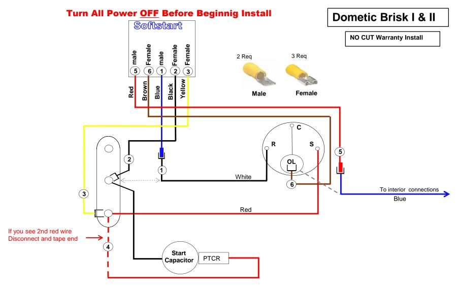
Route Blue, Black and Yellow Softstart wires into electrical box, Then Crimp disconnects on ALL Softstart wire as indicated in Softstart drawing above
