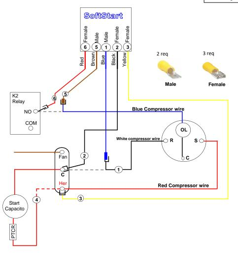
Route ALL softstart wires into Electrical box, then crimp disconnects as shown in softstart drawing above
