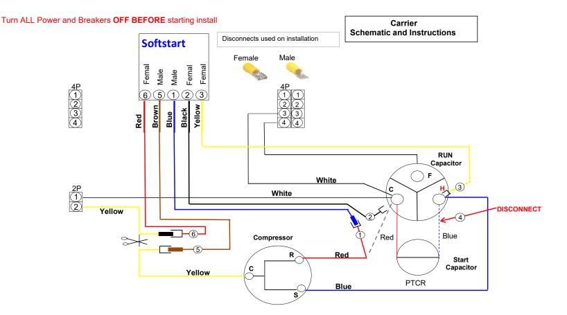
Begin by routing ALL Softstart wire into elcetrical box, Then crimp disconnects on wires as shown in Softstart box above
